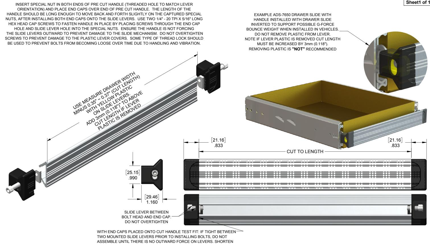
EXTRUSION IF NEEDED. HANDLE SHOULD HAVE 0.010" TO 0.030" FREE PLAY BETWEEN END CAPS AFTER BOLTING IN PLACE.
