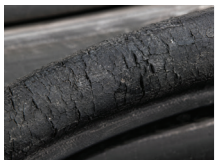
Cracked or flattened weather seals
